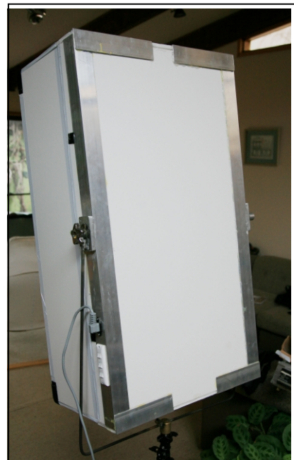
Back of unit showing aluminium angle strengthening members and mounting yoke.
